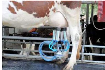
Shashi Kumar said a farmer could milk 25 cows in less than two hours. The milking system is equipped with sensors to generate data regarding body temperature of a cow, the quantity of milk produced and detection of breast infections.
